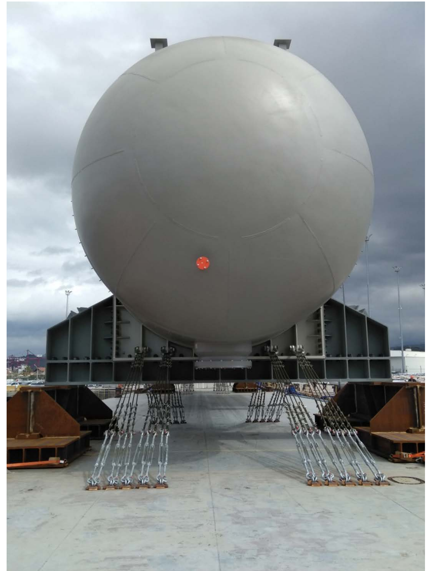
Figure 10: Example of Pressure vessel seafastening and grillage
