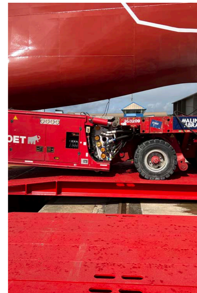
Figure 2 & 3: HMS Venturer being loaded-out by SMPT to CD01, onto bespoke grillage
