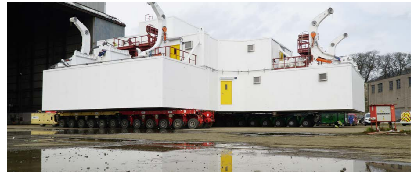
Figure 3: View of SDS module on SPMT's from the South side
